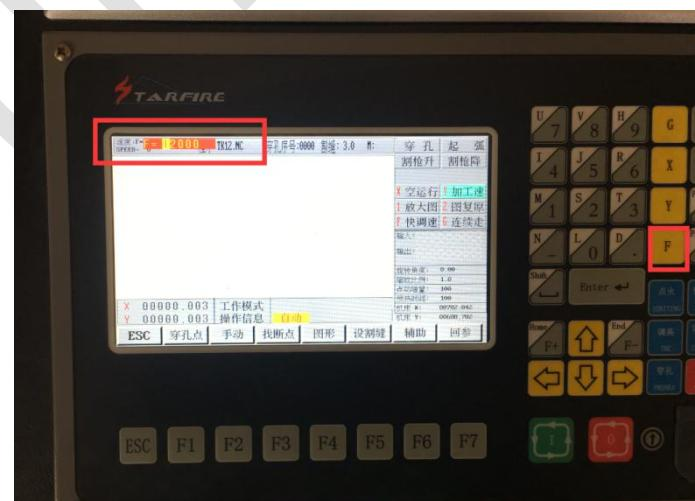
4. The X and Y coordinates are cleared. Write down the X-axis coordinate value of one rotation
