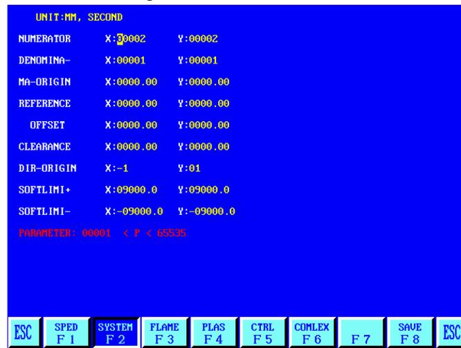
Electronic gear molecular /denominator - electronic gear molecules and the ratio of the denominator is the pulse equivalent, unit microns, converted to X 1000 mm. Molecular < 65535, denominator < 65535.
