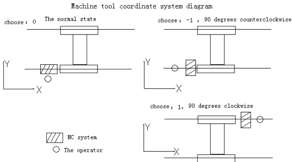
Metric system: 0/ inch metric: 1 choice = metric: 0: length parameters, speed, and the value, the coordinates are metric unit (mm). Can finish English program (G20), but the display is a metric unit (mm).
