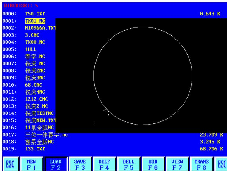
Transfer into the program, select the call in the user program in the program, the system will be an existing program, displayed in a tabular form, and the cursor stays on the program name. Move the cursor keys to select different programs. After press enter, the selected program loading process editor area. If you press "F7", graphic displays of the program. Press "ESC" to give up to function.
