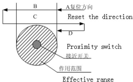
**Section A: to reset speed fast forward.**
