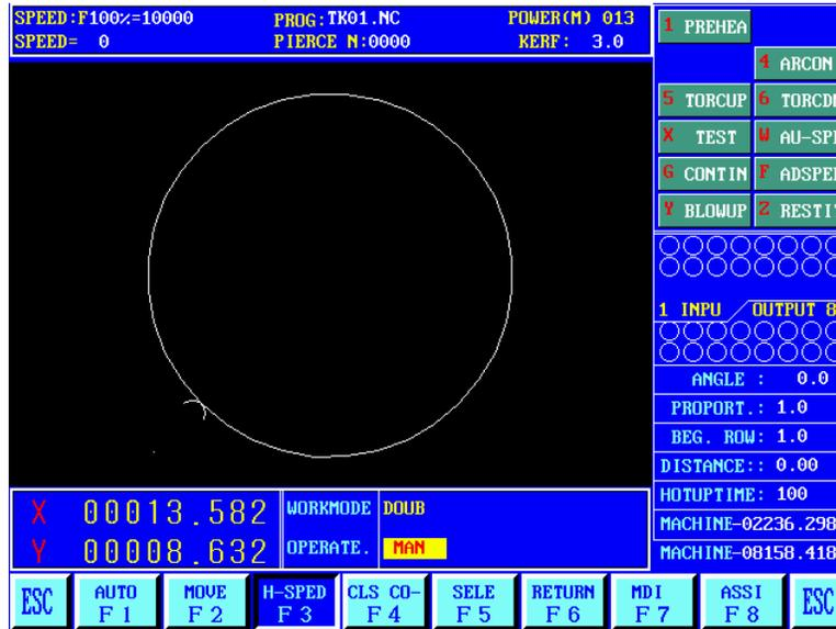
4.1 manually interface manually interface display with automatic mode. Difference in the value of the ratio of the manual, it affects the manual operation, back to the speed, movement speed, etc. Directly on the screen press [F] speed can be set. There are some special operation manual modes.
