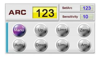
ARC: show the actual arc voltage value after arc strike, 000 is for no arc voltage value.
