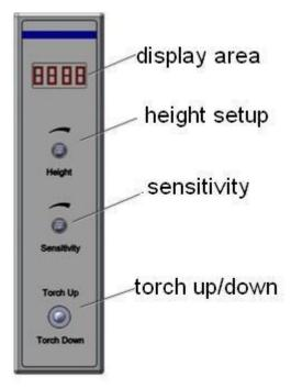
In main interface, press Sensitivity, initial location tests. Press Height to adjust parameters, A is for location height, press Height to be back.
