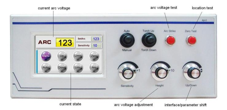
a. Check basic parameters setup of first use
